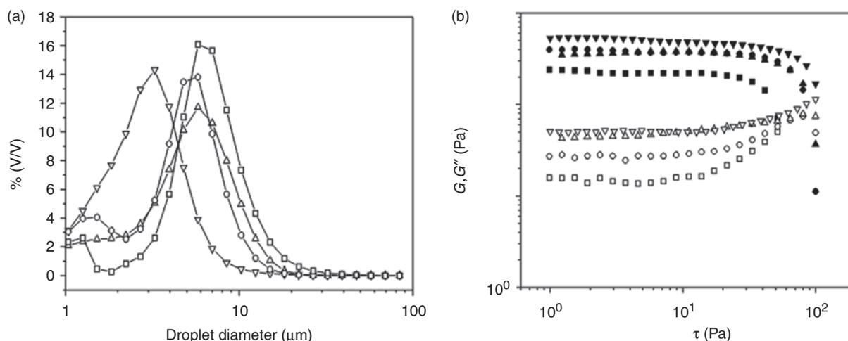
**Figure 4.** (a) DSD and (b) stress sweep (at  $\omega = 6.28$  rad/s) for emulsions processed at 20,500 rpm containing different egg yolk concentrations (2, 3, 4, 5 wt%). (a) ( $\square$ ) 2%; ( $\circ$ ) 3%; ( $\triangle$ ) 4%; ( $\nabla$ ) 5%. (b) ( $\blacksquare$ )  $G'$  ( $\square$ )  $G''$  2%; ( $\bullet$ )  $G'$  ( $\circ$ )  $G''$  3%; ( $\blacktriangle$ )  $G'$  ( $\triangle$ )  $G''$  4%; ( $\blacktriangledown$ )  $G'$  ( $\triangledown$ )  $G''$  5%.
