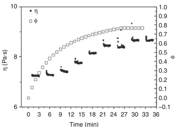
**Figure 2.** Evolution of oil volume fraction and viscosity at  $100 \text{ s}^{-1}$  along the emulsification process at 20,500 rpm for a system containing 75 wt% oil (0.215 mL/s) and 3 wt% yolk.
