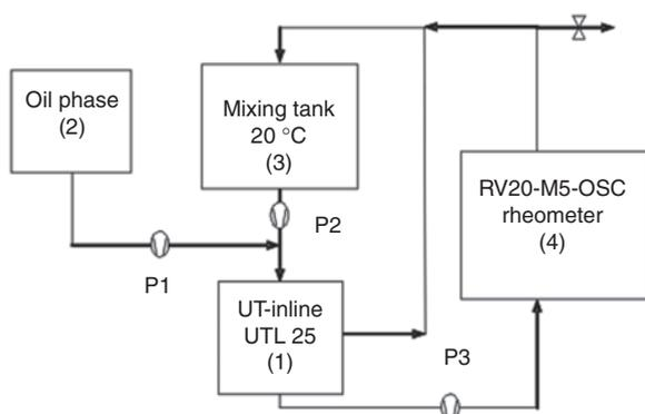
**Figure 1.** Flow diagram for the emulsifying device.
