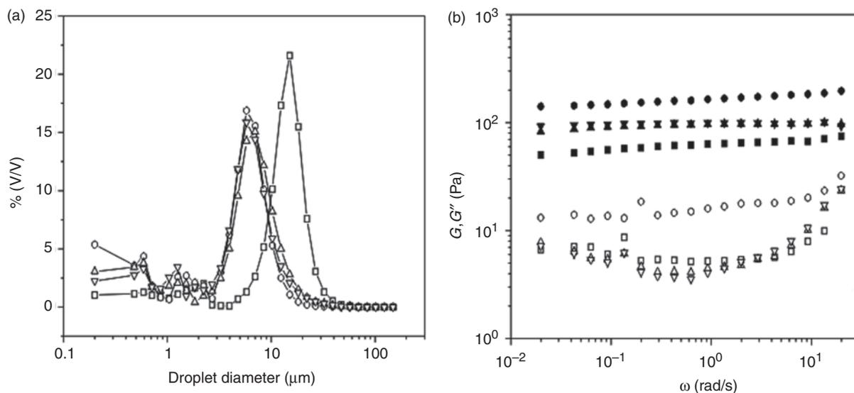
**Figure 5.** (a) DSD and (b) mechanical spectra for emulsions stabilized by 3 wt% egg yolk at different rotation velocities ( $\square$ ) 8,000 ( $\diamond$ ) 13,500, ( $\triangle$ ) 20,500; ( $\nabla$ ) 24,000. (b) ( $\blacksquare$ )  $G'$  ( $\square$ )  $G''$  8,000 rpm, ( $\bullet$ )  $G'$ ; ( $\circ$ )  $G''$  13,500 rpm, ( $\blacktriangle$ )  $G'$ ; ( $\triangle$ )  $G''$  20,500 rpm ( $\blacktriangledown$ )  $G'$ ; ( $\triangledown$ )  $G''$  24,000 rpm.
