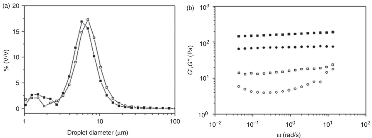
**Figure 3.** (a) DSD and (b) mechanical spectra for an emulsion processed at 13,500 rpm in a semicontinuous device (UTL25) and in a discontinuous batch (UT25). (a) (■) UTL 25; (□) UT 25. (b) UTL25, (■)  $G'$  (□)  $G''$  UT25, (●)  $G'$ , (○)  $G''$  UT25.
