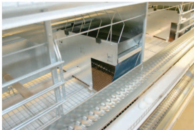
Figure 1. The furnished cage for groups of 8 layers with the nest box located to the right. The litter facility is positioned on top of the nest. During the daily period of access to the litter facility the wire gate was turned down into the litter. No egg belts were present when conducting the trials. Color version available in the online PDF.
