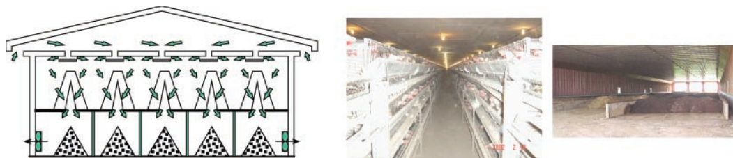
Figure 1. A schematic representation of a high-rise layer house (left) and photos of a manure belt layer house (middle) and manure storage shed (right). Color version available in the online PDF.
